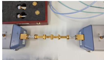
Characterization of waveguide cascade components used in B2B calibration using TRL and UOSM standards
