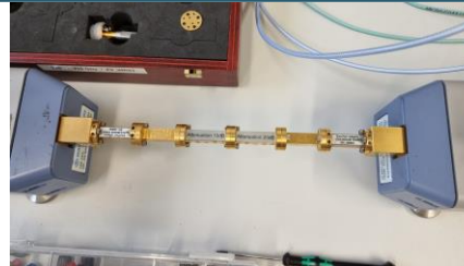
Characterization of different waveguide components and their PDP compared to their electrical length
