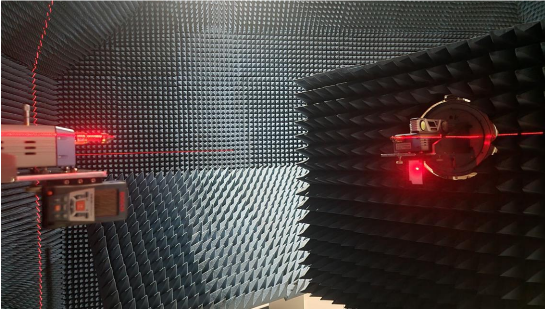
Distance measurement Performed at the antenna scanner room in PTB
