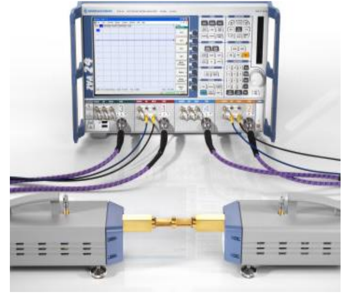
Vector Network Analyzer at WR05, and WR03 frequency bands at PTB
