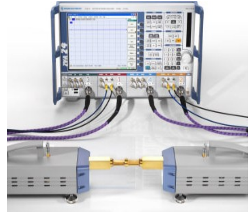
Vector Network Analyzer at WR05, and WR03 frequency bands at PTB from Rohde und Schwarz.
